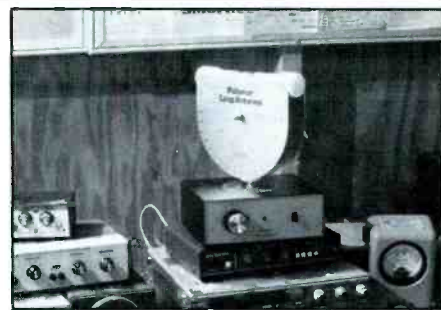
Figure 5— A) Palomar Engineers HF-1 small loop; B) Palomar BCB loopstick. Both are connected to an LA-1 loop amplifier.
